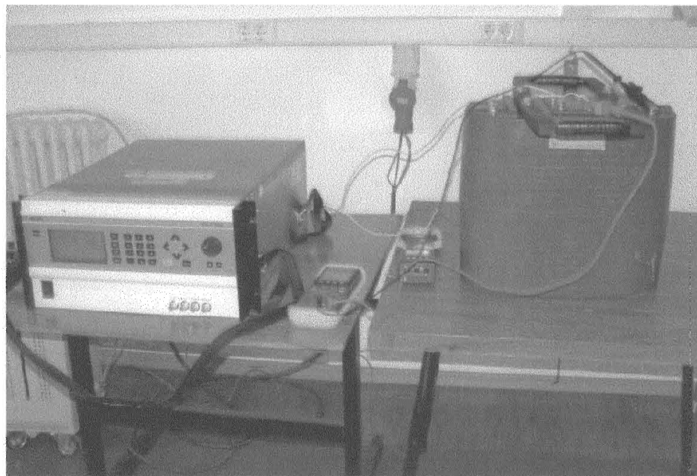
Fig.3 Induced AC withstand voltage test
